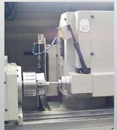
Universal Wheelhead set in Internal Mode
